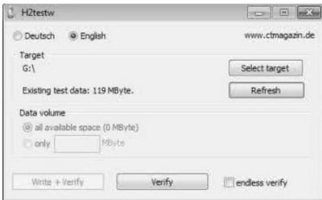
With this software you can verify the capacity and ensure that it works well. The speed measured however depends on both the stick or card and the host device. The tiny capacity of the device in this example resulted in a test time of about a minute; expect much longer times for modern multi-Gbyte devices. Nevertheless, it's worth taking the time to check a new SD card before trying to use it in your camera on a trip to Europe.
